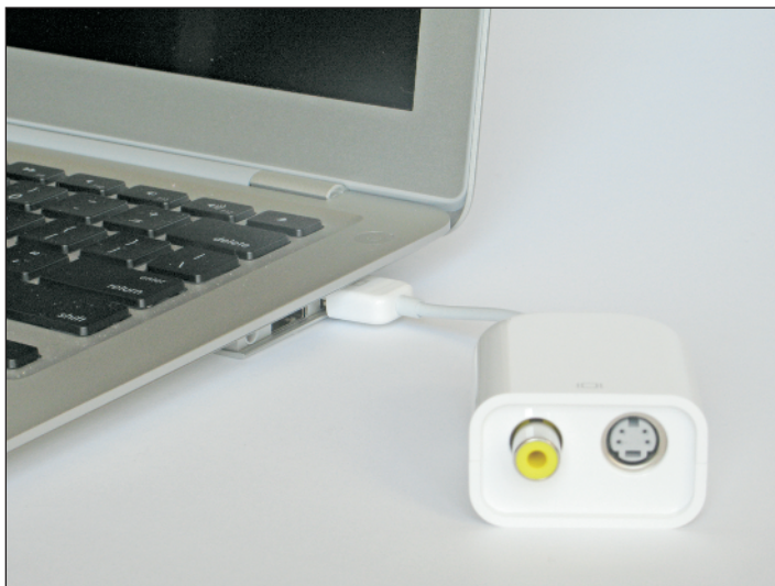
1.8 Use the Micro-DVI to Video adapter to connect your MacBook Air to an external display's Composite or S-Video port.
