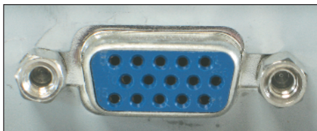
1.5 VGA connectors are standard on CRTs and common on LCDs.
