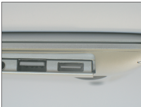
1.1 MacBook Air comes with a Micro-DVI port for connections to external displays.
