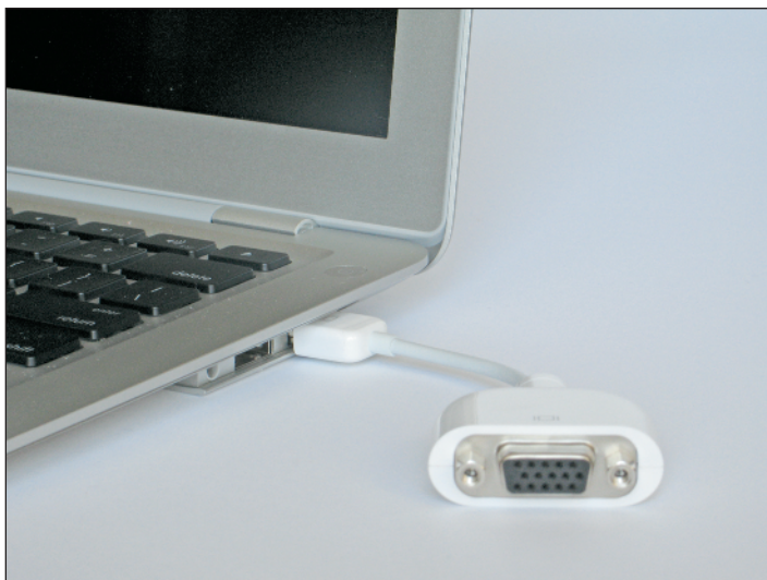
1.6 Use the Micro-DVI to VGA adapter to connect the MacBook Air Micro-DVI port to an external display's VGA port.
