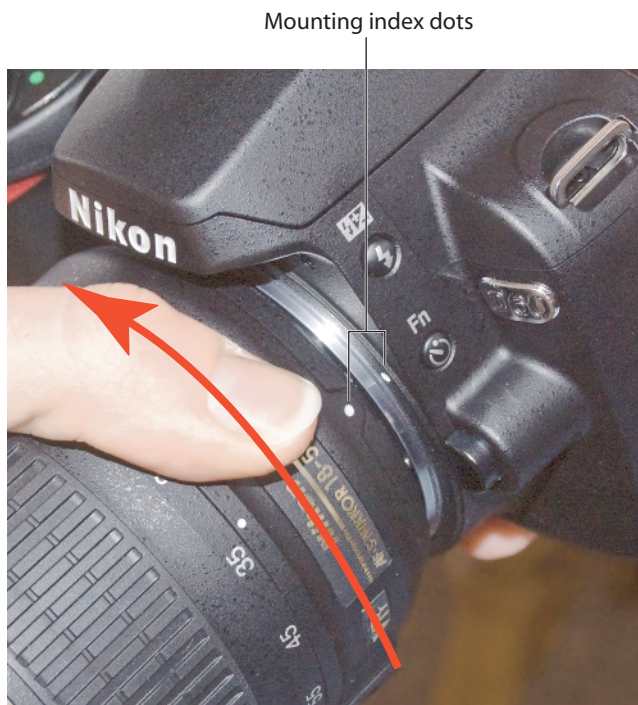
Figure 1-1: When attaching the lens, align the index markers as shown here.
