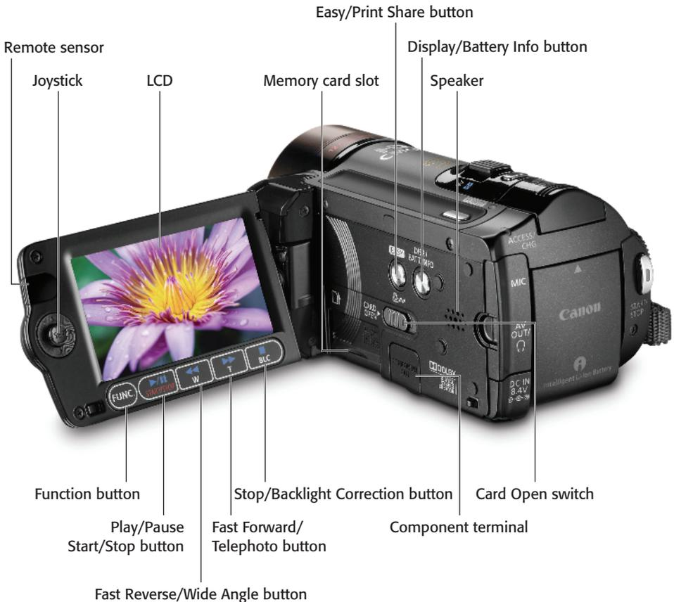
**1.1** The left side of the VIXIA HF10, HF11, and HF100. The VIXIA HF100 body is silver, but the layout is the same.
