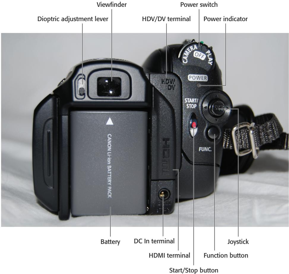
**1.23** The back of the VIXIA HV20 and HV30
