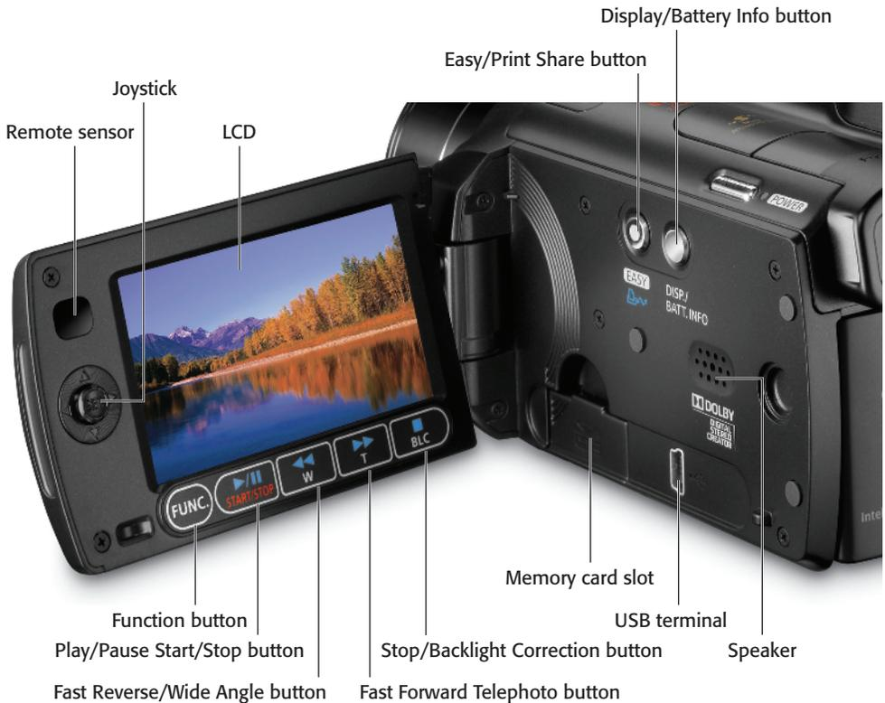
1.6 The left side of the VIXIA HG21. The left side of the VIXIA HG20 is identical.
