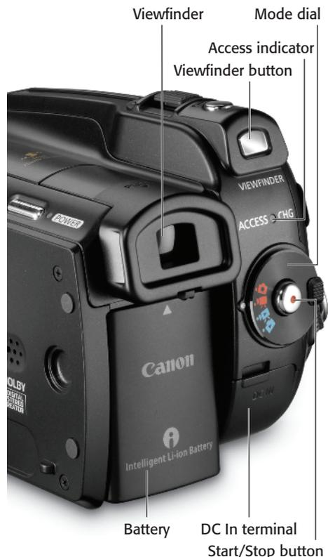
**1.8** The back of the VIXIA HG21. The VIXIA HG20 does not have a viewfinder button like this camcorder, as the VIXIA HG20 has no viewfinder.
