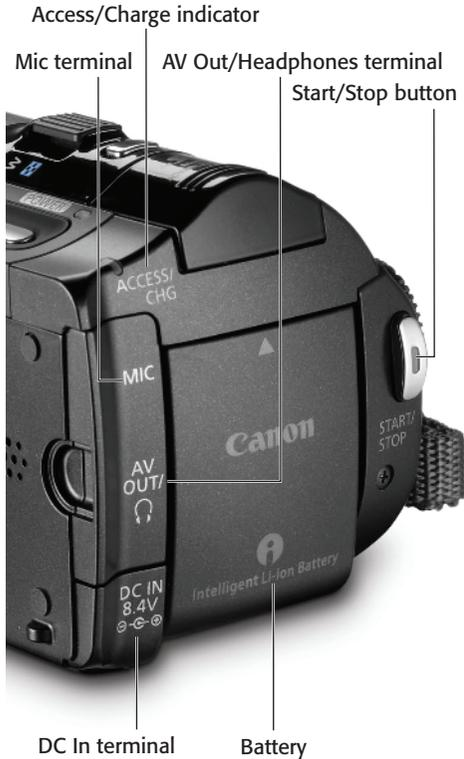
**1.2** The back of the VIXIA HF10, HF11, and HF100. Although the VIXIA HF100 has a silver body, the back of the camcorder is the same.
