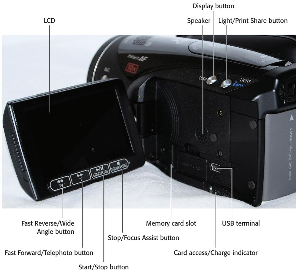
**1.19** The left side of the VIXIA HV30. Other than the silver body, the left side of the VIXIA HV20 is identical.
