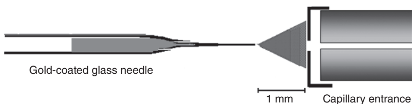
Figure 1.10. Typical instrumental configuration for nano-ESI experiments.
