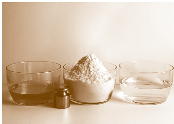
Figure 1.3 Equal weights of (left to right) glucose corn syrup, sifted pastry flour, and water take up different volumes.
