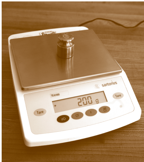
Figure 1.1 Check your scale daily with a known weight to confirm that it is properly calibrated.
