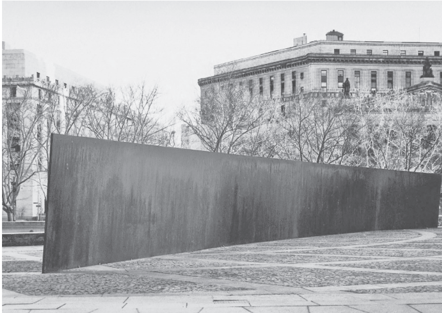
Figure 1–2: Tilted Arc , a sculpture by Richard Serra. Constructed in 1981, this sculpture is a 120-foot- (36.6-m-) long slab of curved steel, 12 feet (3.66 m) tall and 2.5 inches (6.35 cm) thick. It was designed to bisect a public plaza in front of the Jacob Javits Federal Building in Manhattan.
