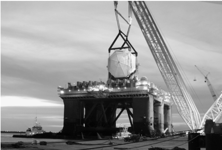
Figure 1.9. SBX-1 array being loaded on board the platform. (Courtesy of Missile Defense Agency History Office.)
