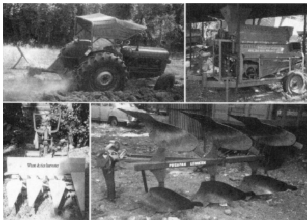
Fig.A.19: Special purpose machines and equipments are devised for various agricultural operations. Clockwise from top left: tractor driven plow, thresher, moldboard plow and wheat and rice harvester.
