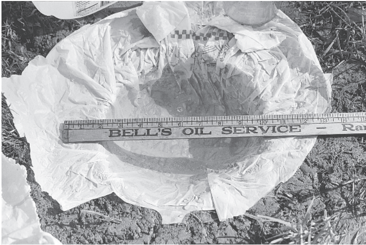
Figure 1.21 Hole is lined with a plastic bag. After the bag has been filled to the top with water, the volume of the water is measured and compared with the weight of the dried soil.
