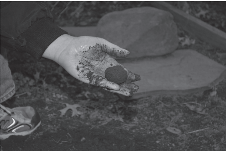
Figure 1.14 Squeeze the soil tightly so that it forms an egg-sized ball.
