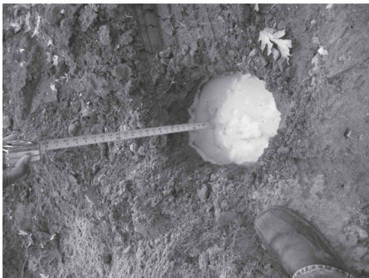
Figure 1.19 Check the depth of the water in the hole on an hourly basis, and record the drop in level in inches.
