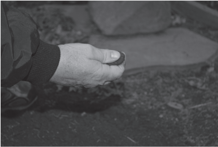
Figure 1.15 Begin to squeeze the soil out between your thumb and forefinger, forming a ribbon.
