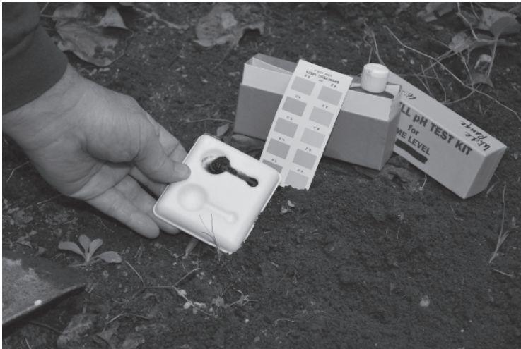
Figure 1.22 A field pH test kit allows preliminary data to be determined.
