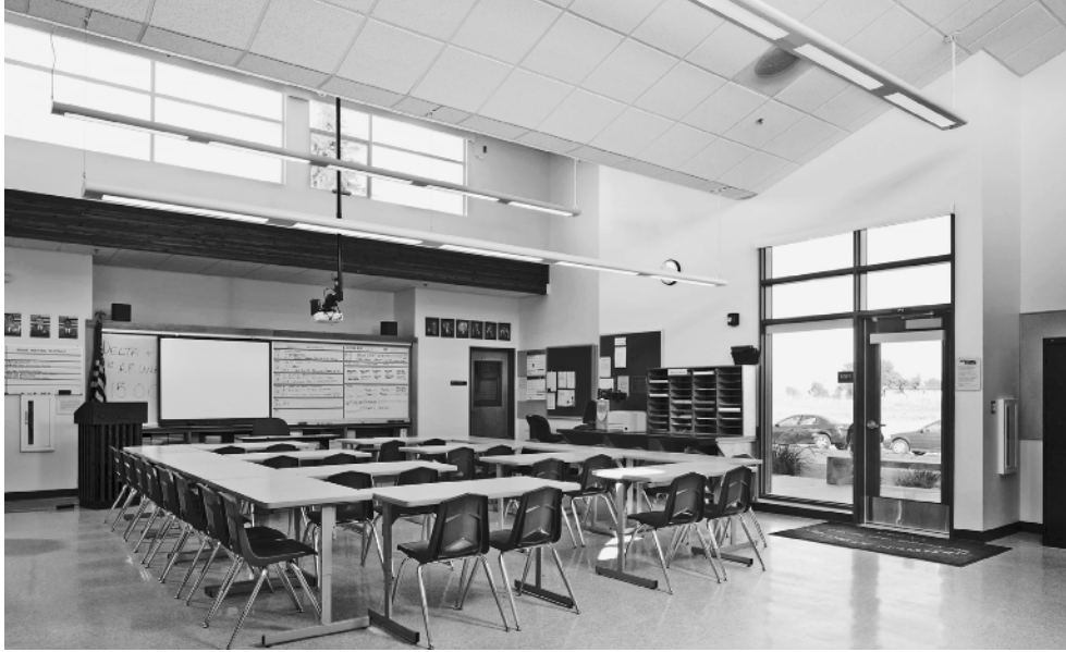
Excellent daylighting and automated window controls make this Vanden High School classroom energy efficient as well as comfortable. Source: Mark Luthringer
