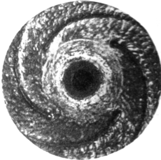
FIGURE 1.6 Erosion-corroded pump propeller.
