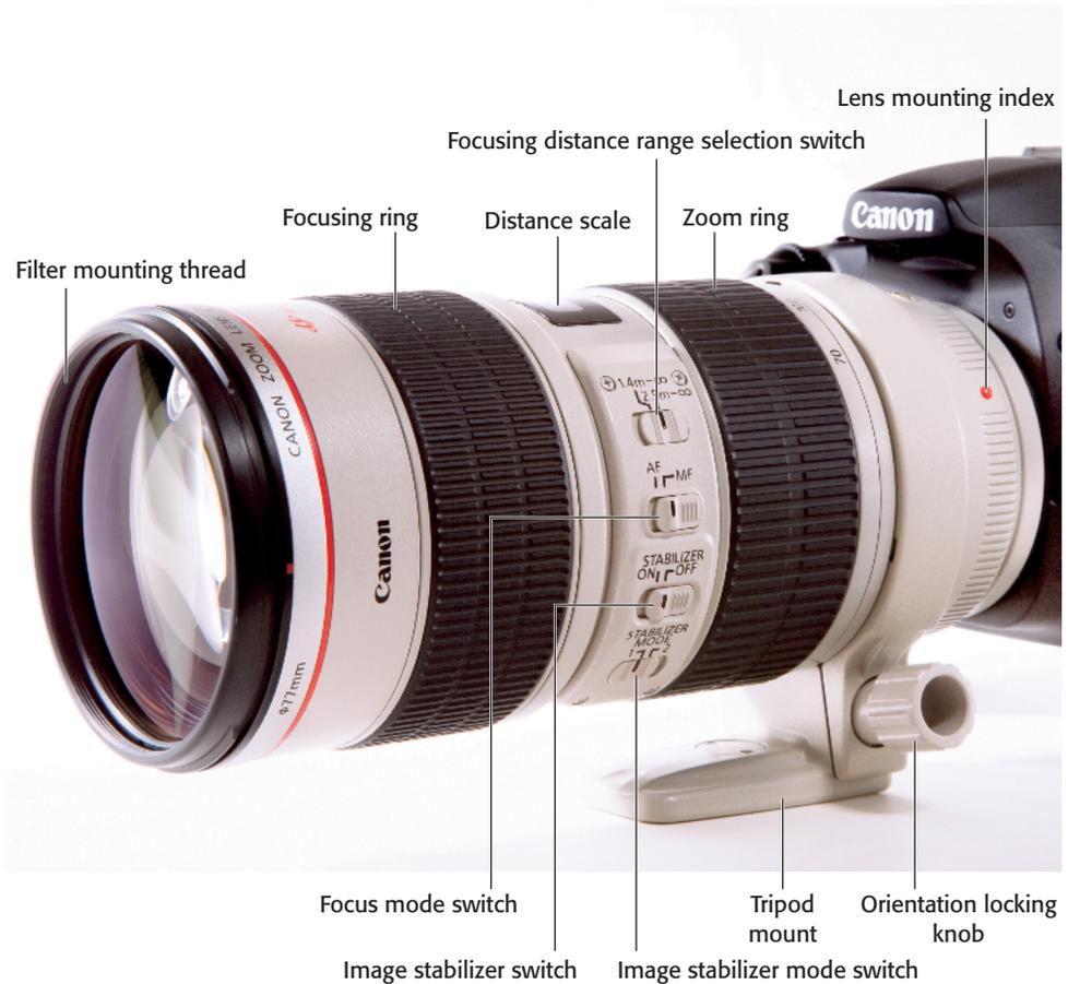
**1.8** Lens controls, as shown on an EF 70-200mm f/2.8L IS USM lens
