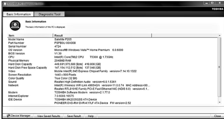
**Figure 1-6:** Testing this Toshiba laptop model, I excluded the dial-up modem and told the software not to bother testing the floppy disk because it's not there.
