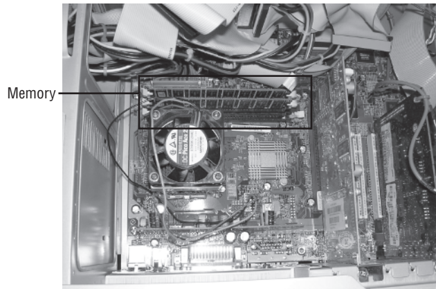
FIGURE 1.29 Location of memory within a system
