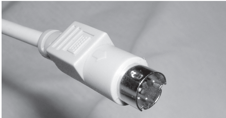
FIGURE 1.54 A PS/2 keyboard cable
