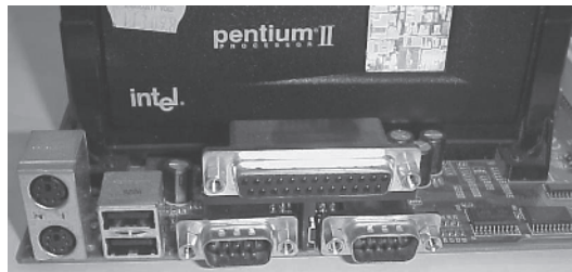
FIGURE 1.21 Built-in ports on a motherboard
