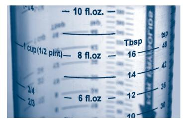
**Equivalent volumes.** One cup, ½ pint, 8 fluid ounces, 16 tablespoons, and 48 teaspoons are all equivalent volumes. Note: This measuring device is correctly marked in fluid ounces. Many volume measuring devices are marked in ounces, which could potentially be confusing. A person using such a device must know it means fluid ounces by volume.
