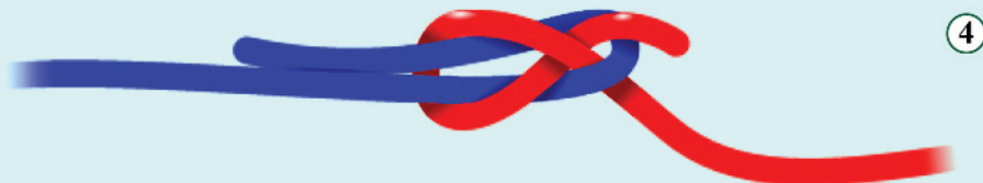
Two lines joined by a sheet bend.
