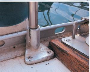
➤ Deck works and fittings. Deck fittings are an authentic disaster. Except for the cockpit winches, which are in a reasonable condition, all the rest is old, broken down or jammed (if not all three at once). A complete update is essential.
