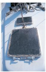
➤ Hatches and companions. As you would expect after almost thirty years of exposure to the elements, the plexiglass of her front windows has become completely glazed, to the point where they are almost opaque. These will have to be replaced, as will the boat's different hatches, including weather seals and badly worn fittings.
