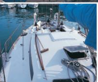
➤ Painting the hull and deck. When it comes to fixing up a boat there are few jobs that work as effectively as a good coat of paint on hull and deck. Samba's gelcoat, thoroughly coarsened, lacking shine and with the wounds of twenty years of service is just crying out for this to be done.
