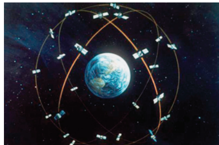
Artwork courtesy of US Dept of Defense Simplified GPS satellite constellation
