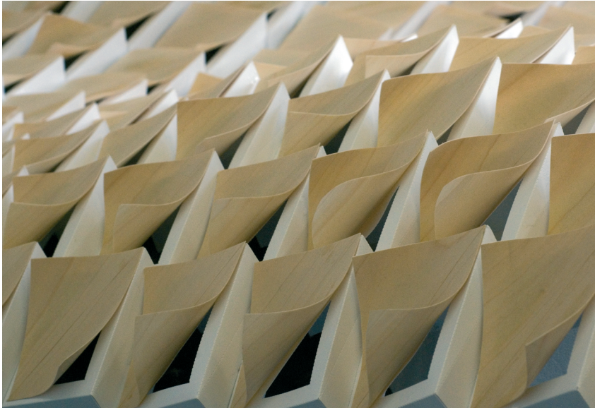
Responsive surface structure that instrumentalises moisture-content activated shape changes of timber components. See 'Material Performance' on page 34.
