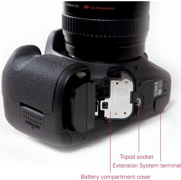
**1.7 EOS 7D bottom-of-the-camera components shown with the LP-E6 battery pack**
