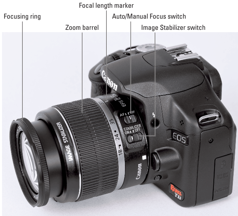
Figure 1-3: Set the focusing switch to MF before turning the manual focus ring.
