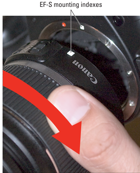
Figure 1-2: Place the lens in the lens mount with the mounting indexes aligned.
