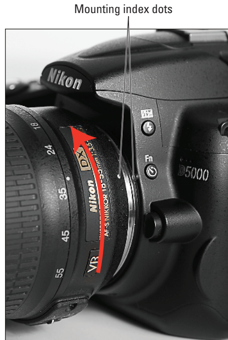
Figure 1-1: When attaching the lens, align the index markers as shown here.
