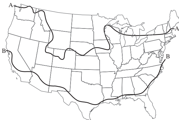
Figure 1.5.3.1-1 Termite damage in the continental United States. A, northern limit of recorded damage done by subterranean termites; B, northern limit of damage done by dry-wood or non-subterranean termites. (From Wood Handbook[34].)
