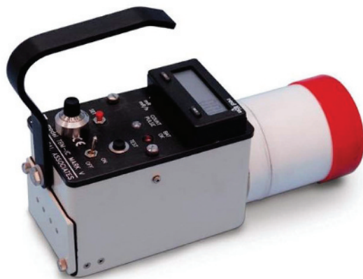
Figure 1.55 A “cutie pie” portable survey meter. The scale of the meter is calibrated to read directly in units of milliroentgens per hour, with a range switch that decreases the sensitivity of the meter by factors of 10.
