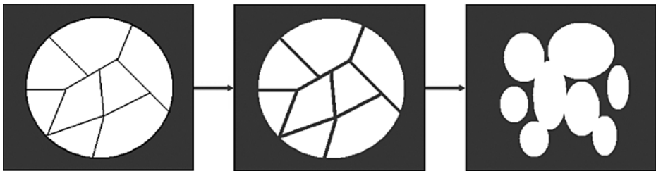
Figure 1.12. Schematic of secondary rearrangement for polycrystalline particles during liquid-phase sintering.
