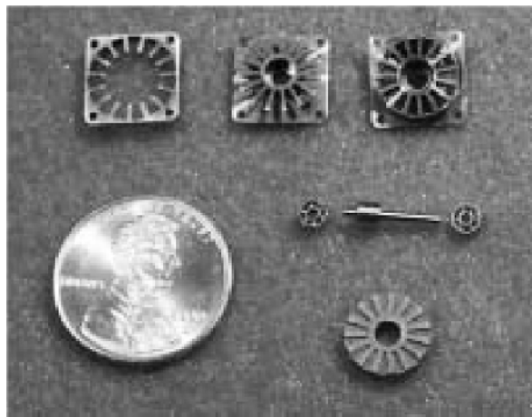
Figure 1.11 Meso-scale stepper motor (10 mm \times 10 mm \times 5 mm) machined by Micro-EDM process. Source: Courtesy of Sandia Manufacturing Science and Technology Center.
