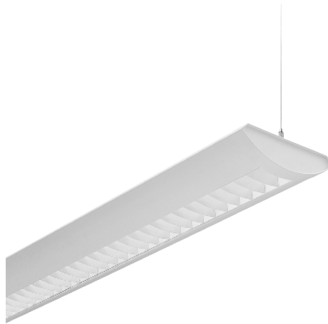
Figure 1-13b Direct/indirect fluorescent luminaire combines the softened effect of indirect lighting with a direct light component. (Provided by Philips Lightolier.)
