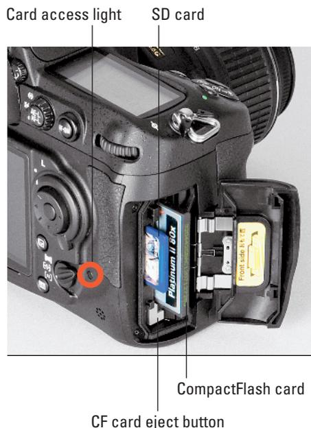
**Figure 1-15:** Insert cards with the labels facing the back of the camera.
