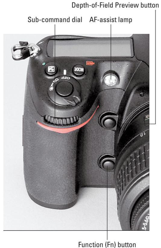
**Figure 1-23:** You can assign the Function button to perform a variety of operations.
