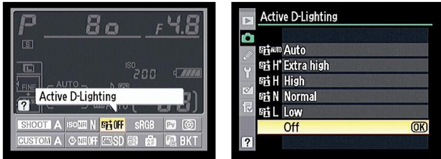
**Figure 1-12:** Press the Info button while the Information screen is displayed to gain quick access to the settings at the bottom of the screen.
