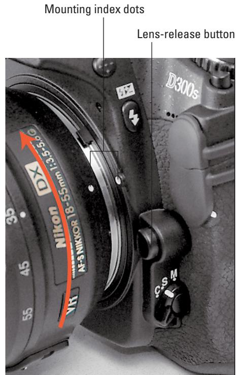
**Figure 1-3:** When attaching the lens, align the index markers as shown here.
