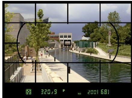
**Figure 1-33:** The viewfinder grid is another aid for ensuring that the horizon is level in the frame.
