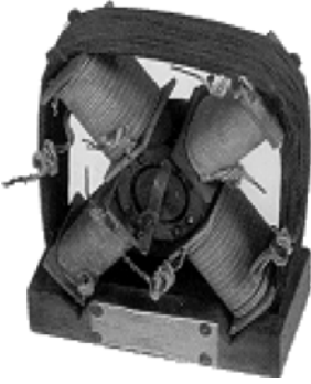
Figure 1.1 Induction machine at early stage of development.
