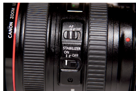
Figure 1-8: Slide this switch to enable image stabilization.
