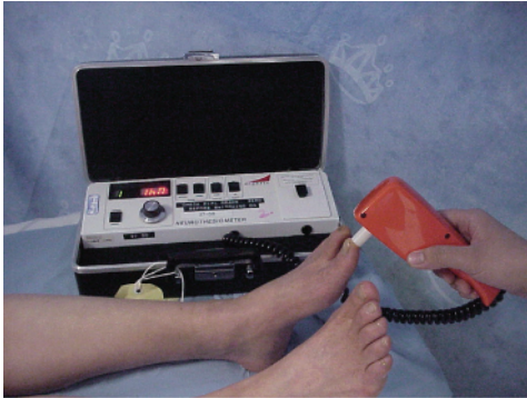
Fig. 1.6 A neurothesiometer is a device that delivers a vibratory stimulus which increases as the voltage is raised.
