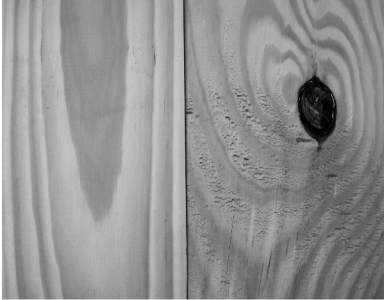
Figure 1.6 Two pieces of timber: one straight-grained, showing smooth surface and another with a grain problem, showing a 'splintery' surface
