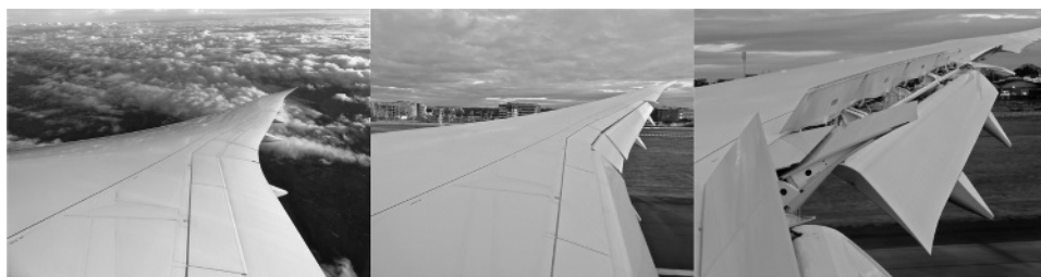
Figure 1.2 Three wing geometries packaged into one and able to morph from one to another: the trailing edge of the wing of a Boeing 787-8 airliner in (from left to right) cruising flight, final approach and touch-down (photographs by A. Sóbester).
