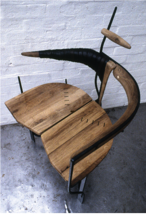
left: Sixteen*(makers)' first commission, a bespoke chair made at Sunbury Workshops, Shoreditch, London EC1, 1995. Materials: oak, leather, 35 mm (1.38 in.) mild steel. Photograph: Bob Sheil. © sixteen*(makers).
