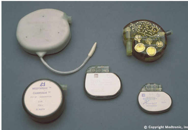
Figure 1.4 Early implantable single chamber device to current dual chamber Kappa. (Source: Reproduced with permission of Medtronic, Inc.)
