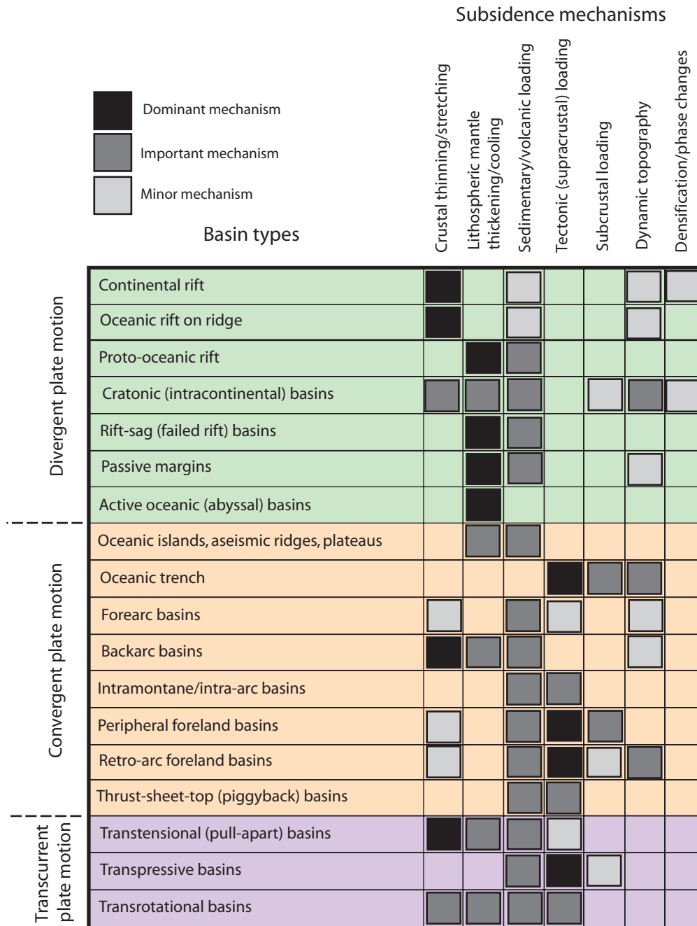
Fig. 1.16 Matrix of main basin types and the principal mechanisms of subsidence (adapted from Ingersoll & Busby 1995 and Ingersoll 2011). Note that subsidence mechanisms operate in more than one basin type, and that several mechanisms may operate in a single basin type. Some basins are ‘polyhistory’ and may pass through phases characterised by different sets of mechanisms.
