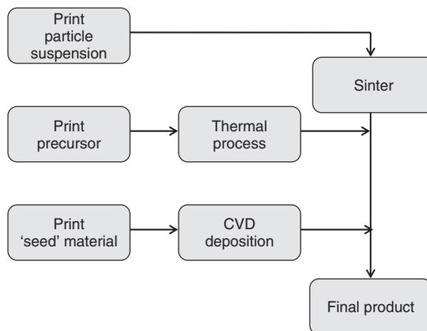
**Figure 1.3** Process routes by which inkjet printing can be used to deposit ceramics.
