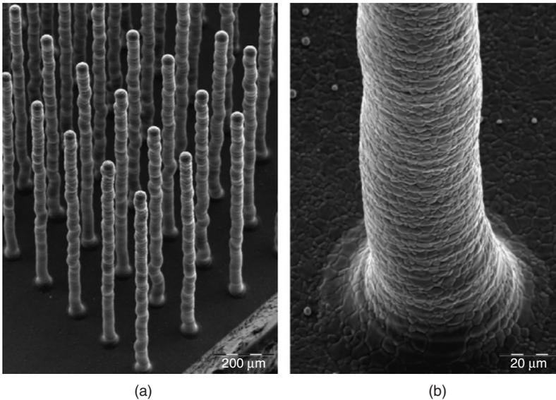
**Figure 1.9** (a,b) Sintered titania pillars formed by inkjet printing (Reproduced with permission from Lejeune et al. (2009) Copyright (2009) Elsevier Ltd.).
