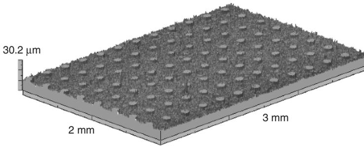
**Figure 1.11** Steel surface patterned by inkjet masking followed by etching. The circular masked regions are  $60\ \mu\text{m}$  in diameter (Reproduced with permission from Costa and Hutchings (2008). Copyright (2008) Society for Imaging Science and Technology).
