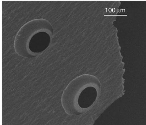
**Figure 1.13** Example of polymer micro-sieve made by inverse inkjet printing (Reproduced with permission from Jahn et al. (2009). Copyright (2009) American Chemical Society).
