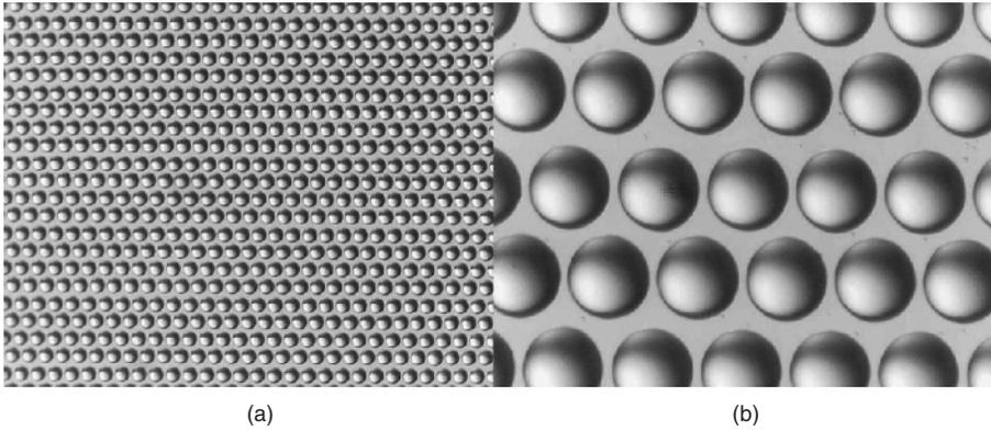
**Figure 1.10** (a,b) Portion of array of 200 000 polymer lenses, each  $104\mu\text{m}$  diameter, formed by inkjet printing (Reproduced with permission from Wallace et al. (2006). Copyright (2006) SMTA Courtesy of MicroFab).
