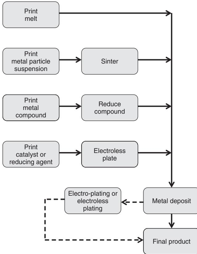
**Figure 1.2** Process routes by which inkjet printing can be used to deposit metals.
