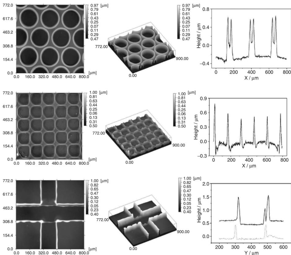
**Figure 1.12** Examples of features etched into a polymer surface (polystyrene) by inkjet printing of solvent droplets (Reproduced with permission from De Gans *et al.* (2007). Copyright (2007) Royal Society of Chemistry).
