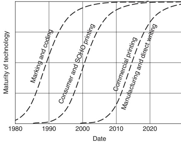
**Figure 1.1** The applications of inkjet technology have developed in three waves: initially for marking and coding, followed by desktop printing of text and graphics in the home and small office environment and, currently, increasing use in commercial printing and manufacturing.
