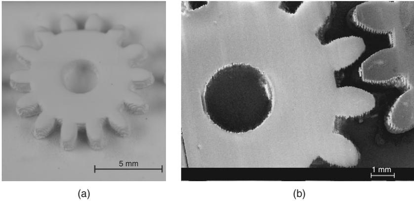
**Figure 1.8** Silicon nitride gearwheels printed by thermal drop-on-demand inkjet: (a) green (as-printed, unsintered) and (b) sintered components (Reproduced with permission from Cappi et al. (2008) Copyright (2008) Elsevier Ltd.).
