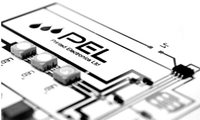
**Figure 1.6** Conducting tracks, 0.5 mm wide, made by drop-on-demand printing of silver nanoparticle ink onto a ceramic substrate, followed by thermal sintering (Courtesy of Printed Electronics Ltd.).
