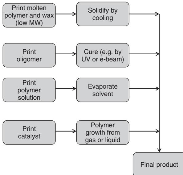
**Figure 1.4** Process routes by which inkjet printing can be used to deposit polymers.
