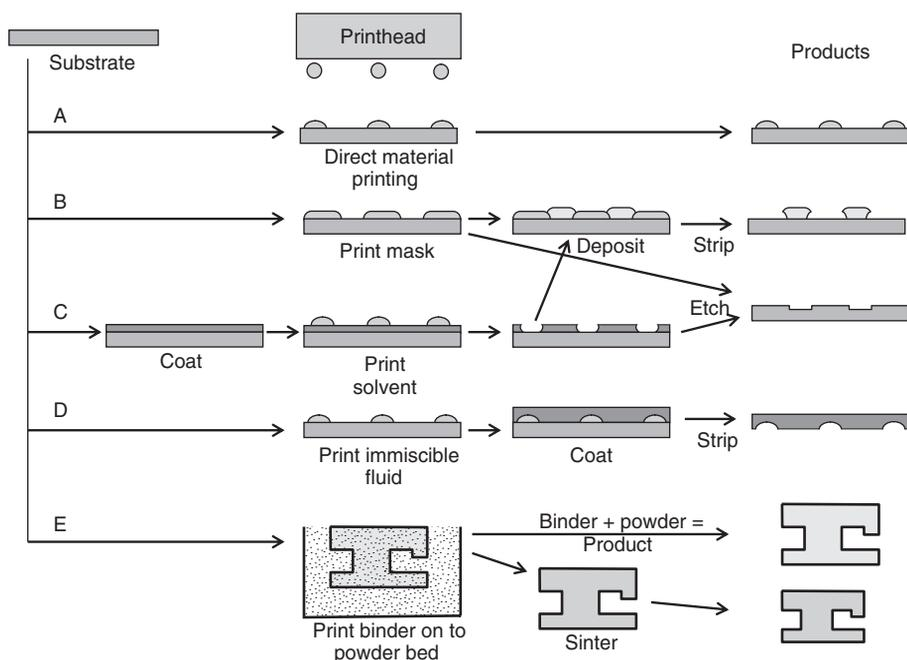
**Figure 1.5** Classification of process routes by which inkjet printing can be used to create structures: (A) direct material printing; (B) printing of a mask followed by material deposition or etching; (C) inkjet etching; (D) inverse inkjet printing and (E) printing onto a powder bed (See plate section for coloured version).
