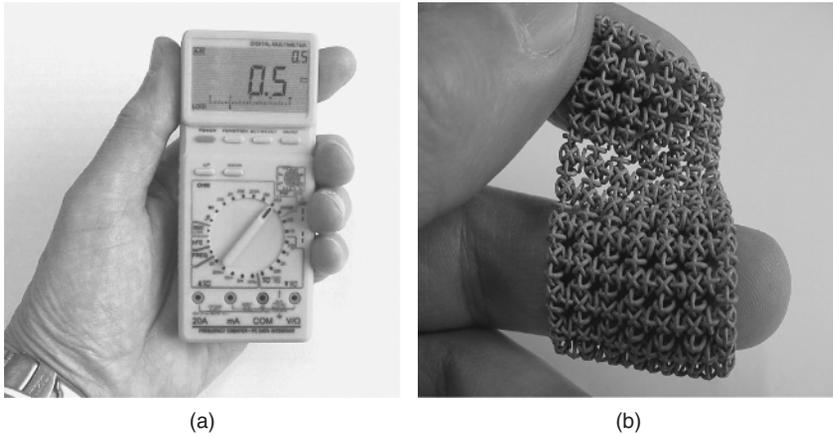
**Figure 1.14** Examples of parts made by printing onto a powder bed: (a) model of an electronic multimeter, made by printing binder onto ceramic powder by the Z-Corp™ process, and (b) stainless steel mesh, sintered after printing onto metal powder by the f cubic™ process.
