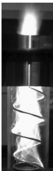
Figure 1.11 Gliding arc discharge stabilized in the 'tornado' gas flow.
