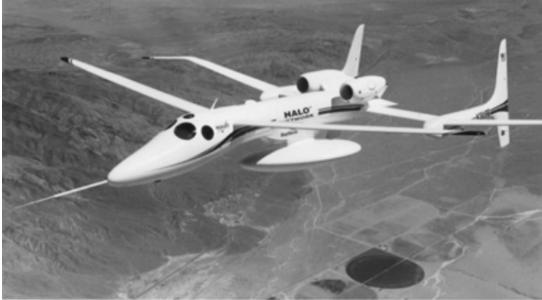
Figure 1.3 The Angel Technologies – HALO plane with antenna pod below. Reproduced from © Angel Technologies
