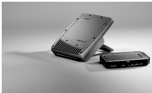
Figure 1.4 A broadband mobile user terminal for packet or circuit-mode operation. Courtesy © Nera Satcom.
