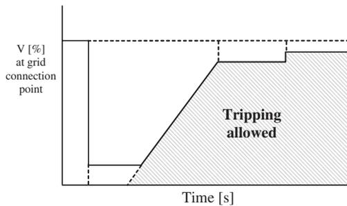
**Figure 1.11** Typical shape of Fault Ride Through capability plot (after Great Britain and Ireland Grid Codes; ESB National Grid, 2008; National Grid, 2008)
