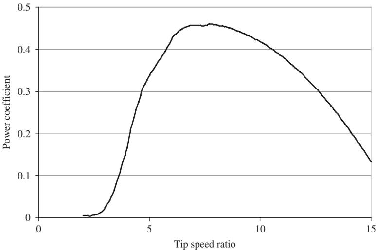
**Figure 1.4** Illustration of power coefficient/tip-speed ratio curve,  $C_p/\lambda$
