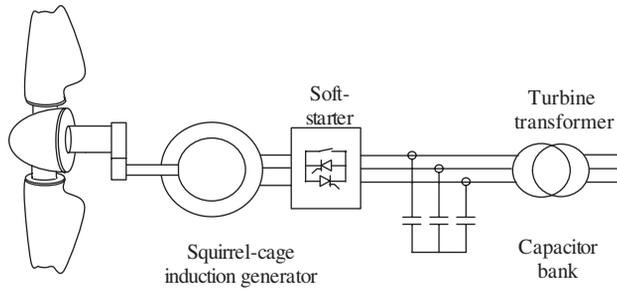
**Figure 1.6** Schematic of a fixed-speed wind turbine
