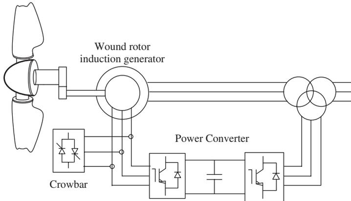
**Figure 1.7** Typical configuration of a DFIG wind turbine
