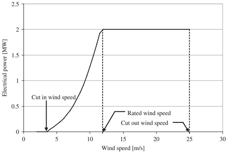
**Figure 1.5** Power curve for a 2 MW wind turbine
