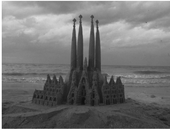
Figure 1.3 Capillary hardening – a little water added to initially dry sand gets trapped between the sand grains by capillary bridges. Being strongly depressurized, this water sticks the grains together and gives cohesion to damp sand, making possible this beautiful reproduction on the beach of Gaudi's Sagrada Familia (copyright Thierry Joffroy, CRATerre-ENSAG). For a mechanical analysis see Section 10.2.4
