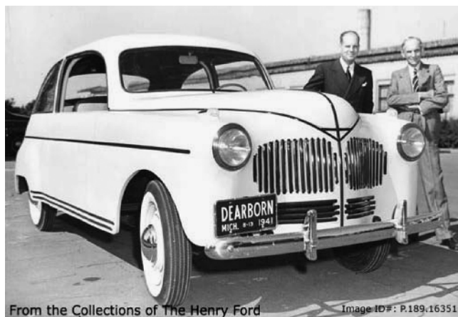
Figure 1.6 A “soybean car” containing biobased materials. Courtesy of The Henry Ford
