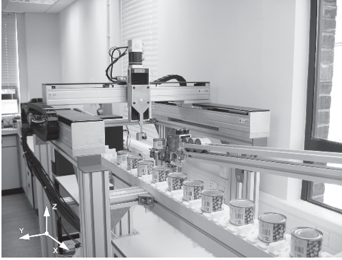
Figure 1.1 A gantry robot for a pick-and-place operation with the axes marked.
