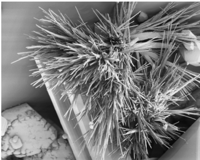
Figure 1.1 Scanning electron micrograph of mullite needles formed hydrothermally in small druses of volcanic rocks of the Eifel mountain, Germany (Reproduced with permission from Mullite by H. Schneider, Fig. 1.3, xvii, Edts. H. Schneider and S. Komarneni, Copyright (2005) Wiley-VCH)
