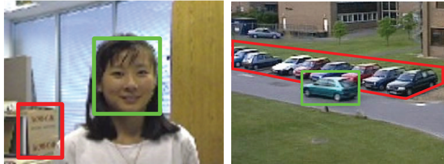
Figure 1.2 Examples of clutter in video tracking. Objects in the background (red boxes) may share similar colour (left) or shape (right) properties with the target and therefore distract the tracker from the desired object of interest (green boxes). Left: image from the Birchfield head-tracking dataset. Right: Surveillance scenario from PETS-2001 dataset.
