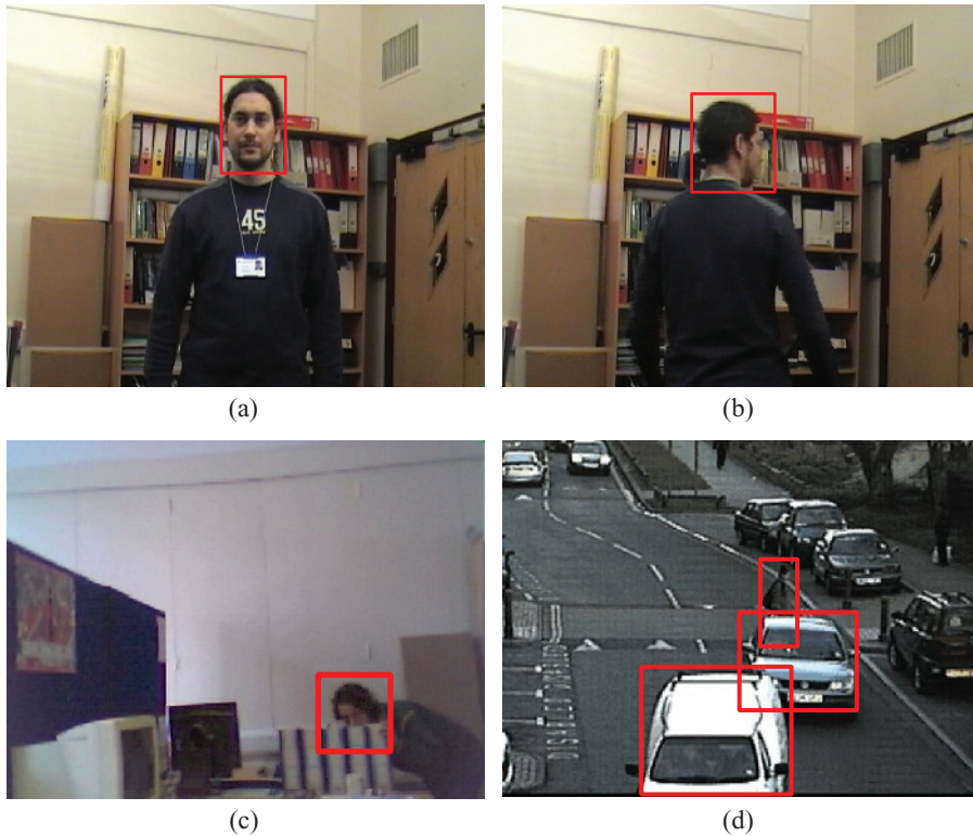
Figure 1.3 Examples of target appearance changes that make video tracking difficult. (a)–(b) A target (the head) changes its pose and therefore its appearance as seen by the camera. Bottom row: Two examples of target occlusions. (c) The view of the target is occluded by static objects in the scene. (d) The view of the target is occluded by another moving object in the scene; reproduced with permission of HOSDB.
