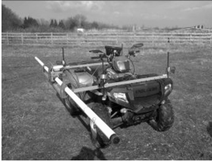
Figure 1.16 Geonics EM-31 mounted on a quad bike. Induced currents will flow in the vehicle as well as in the ground, but should be reasonably constant.
