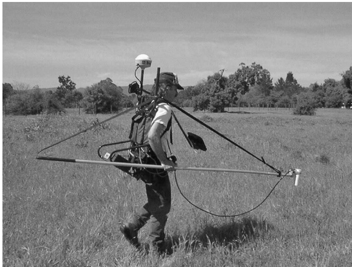
Figure 1.15 Magnetometer coupled to a differential GPS navigation system for continuous profiling. Unless allowance is made in processing for the offset between the GPS and magnetic sensors, anomaly locations will be incorrectly plotted (photo courtesy of Geometrics).
