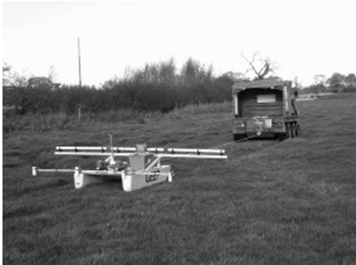
Figure 1.17 Multiple systems mounted on a purpose-built wooden sledge.
