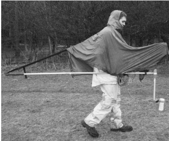
Figure 1.8 The geophysical cape in action. Electronics and observer are both dry, with only the sensor bottle exposed to the elements. The observer can retreat still further, to view the display.
