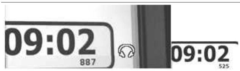
Figure 1.6 Single end-to-end delay measurement of an MPEG-4/AVC video stream from an HD-PVR encoder at a rate of 6.5 Mbps. The delay is (887 - 525 = 362) ms. The delay is measured by taking snapshot images of both the original display (left) and the transmitted video (right) of a running clock.
