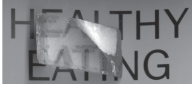
Figure 1.13 The formation of two waves due to the anisotropic properties of calcite.
